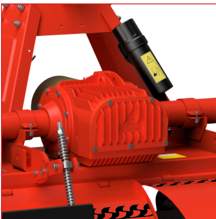
PTO shaft pre-set @1000 rpm
