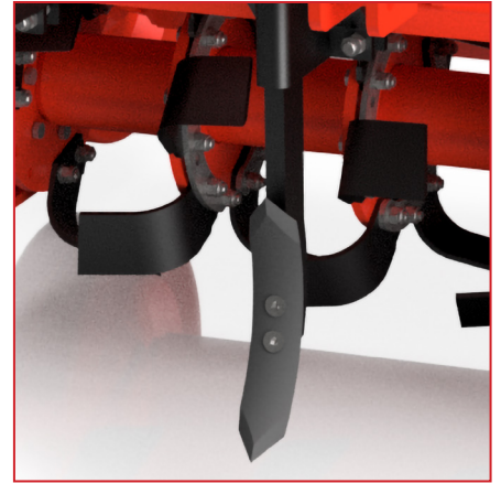
Pair of track eradicators with shear bolt
